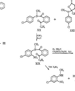
was established by acid hydrolysis to give 4-chloro-2nitro-N-methylaniline and o-benzoylbenzoic acid. Conversion of XIX to the desired dibenzo [b, f] [1,4]diazocine (IV) was effected by reductive cyclization in poor yield.
